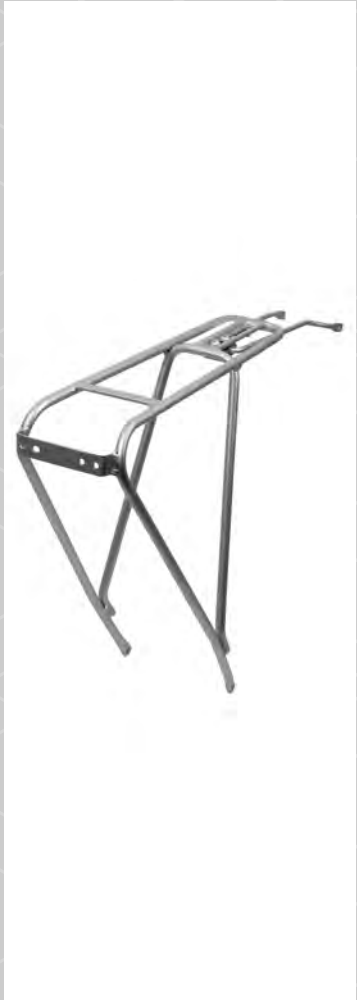
TR-RCR-110 Product: Rear Carrier Size: 28"/27.5"/26"/24"/20" Material: Steel 13x1.2 Tube Features: 50-80mm Bracket Maximum 25kg Colour: Black, Silver
