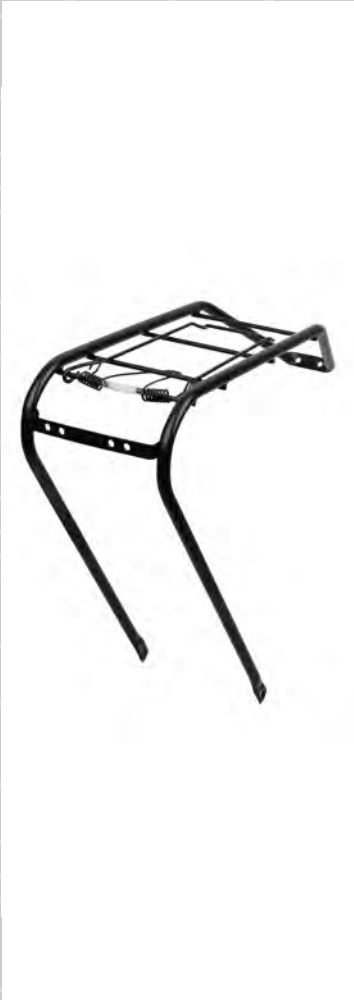
TR-RCR-120 Product: Rear Carrier Size: 28"/27.5"/26"/24"/20" Material: Steel 13x1.2 Tube Features: D-Type With Spring 50-80mm Bracket Maximum 25kg Colour: Black
