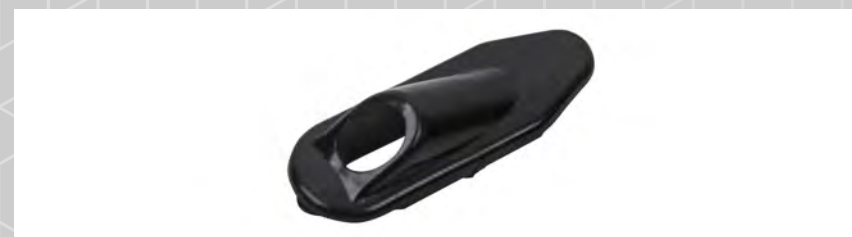
TR-FRP-102 Product: Cable Guide for Top Tube & Down Tube Material: Plastic Compatibility: Thickness of Tube < 1.8mm Slot: 25x6mm Cable hole Ø: 5mm single Colour: Black
