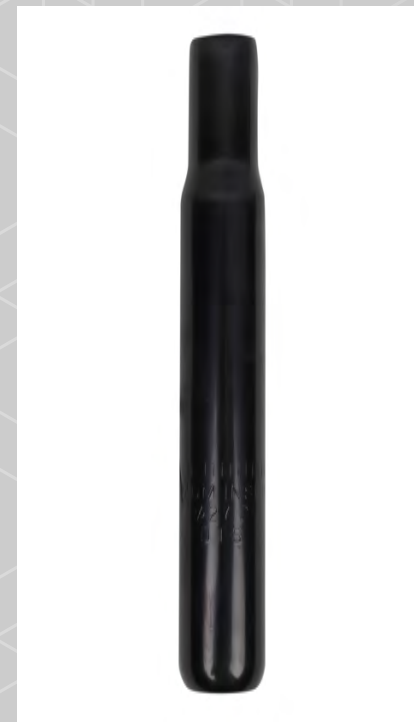
TR-SPT-110 Material: Steel Diameter: Ø25.4/Ø27.2/Ø28.6/Ø30/Ø32/Ø34 Length: 200/250/300/350/400/500 Colour: Black, Silver
