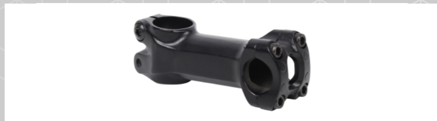
TR-STM-221 Material: Diecast Aluminium Extension: 90mm Barbore: 25.4mm Rise: +7° Steerer: 28.6mm Surface: Sandblasted Black
