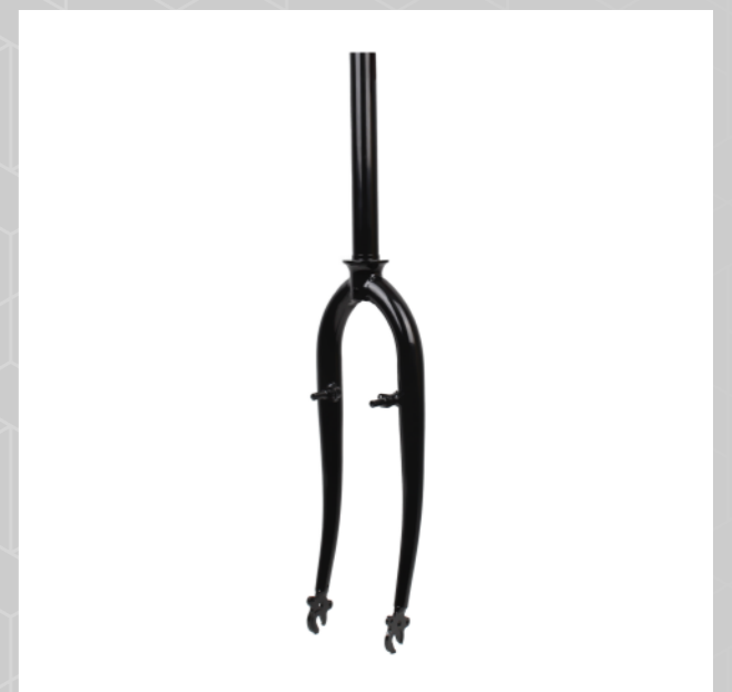
TR-FRK-114 Size: 28" Material: Steel Steerer Tube: 1" or 1 1/8" OLD: 100mm Brake: VBrake or IS Disc Brake Fitting: Double M5 Hole W/Safety Washer Hole Colour: Optional
