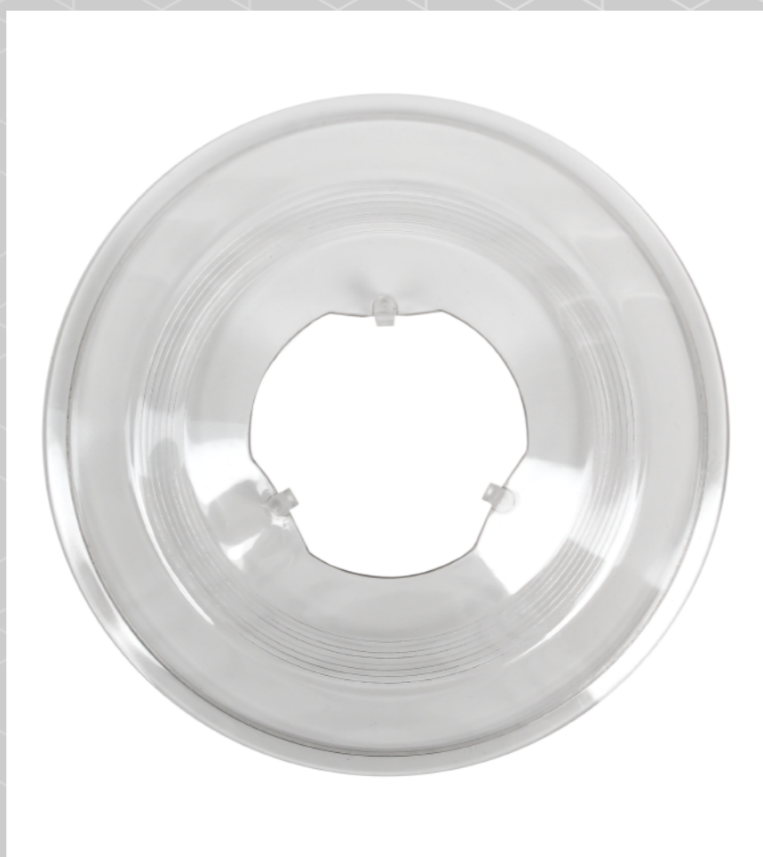
TR-SPP-120 Type: Cassette Hub Type 3 Teeth 36H Compatible Material: PC Outer Diameter Ø: 155mm Inner Diameter Ø: 50mm Colour: Transparent
