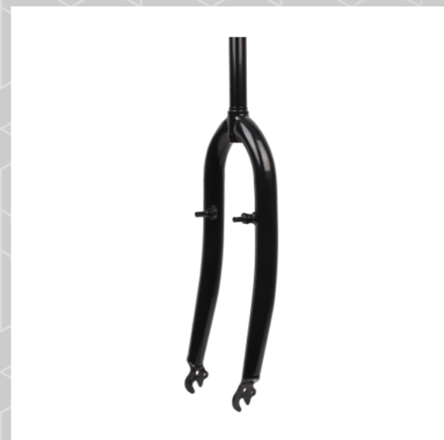
TR-FRK-113 Size: 28" Material: Steel Steerer Tube: 1" or 1 1/8" OLD: 100mm Brake: VBrake or IS Disc Brake Fitting: Single M5 Hole W/Safety Washer Hole Colour: Optional
