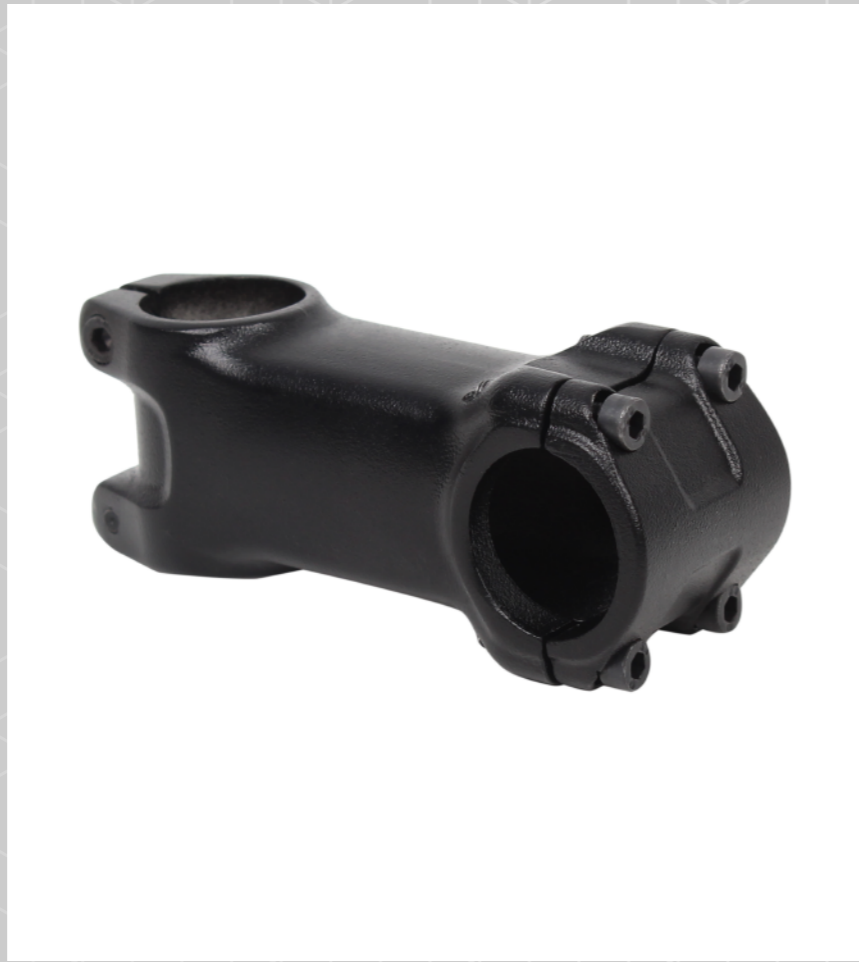
TR-STM-220 Material: Diecast Aluminium Extension: 80mm Barbore: 31.8mm Rise: 3° Steerer: 28.6mm Surface: Sandblasted Black
